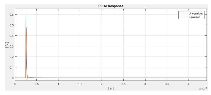
Notice the difference in the pulse response before and after equalization.
