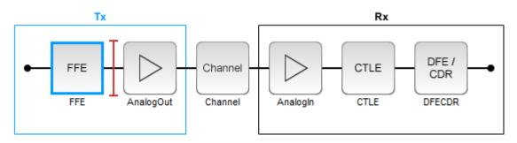
Select the FFE block in the Tx subsystem. In the Block Parameters window, change **Tap weights** from  $[0 \ 1 \ 0 \ 0]$  to  $[0 \ 1 \ 0 \ 0]$ , so that the FFE has one pre tap, one main tap, and two post taps. Leave all other blocks in their default settings.
