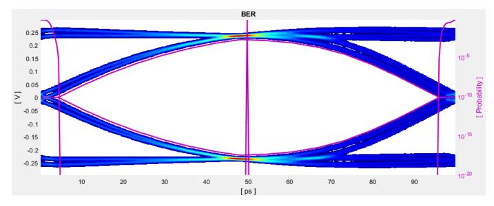
The eye diagram is used to determine the quality of signal integrity. An "open" eye indicates a higher probability of bit recovery. The bathtub curve plots the bit error rate as a horizontal function of the data eye and corresponds to eye width. The contour curve plots the bit error rate as a vertical function of the data eye, and corresponds to eye height.
